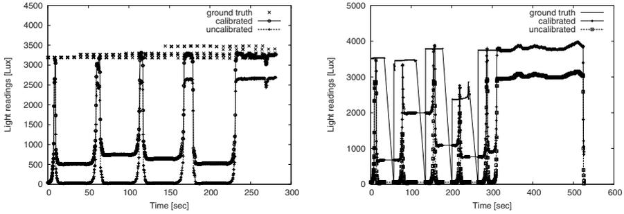
(a) Plot of the calibration performance when a set of five ground truth nodes sit within a  $1m^2$  area. (b) Plot of the calibration performance when the uncalibrated node sequentially encounters five different ground truth nodes.
